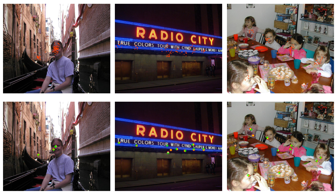
Figure 3: Meanshift fixation detection results on two Judd images. On left is the noisy, subsampled gaze data used for testing. On right are the detected fixations. Red circles indicate ground truth (detected in 240Hz data using code provided by Judd et al. ) and yellow crosses indicate fixations detected in the noisy 30Hz data using our meanshift approach.
