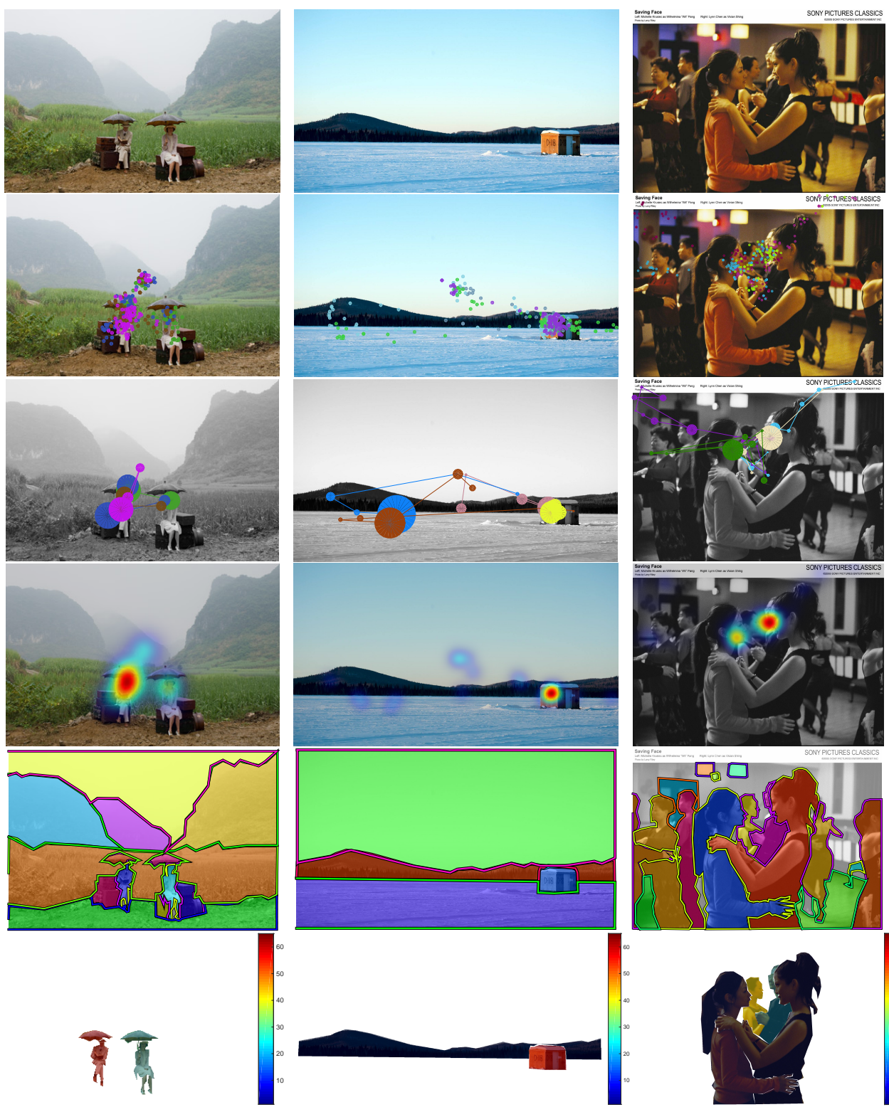
Figure 5: Examples of the image saliency data obtained by our system. In a free-viewing task, users were shown selected images from the SUN database with fully annotated objects. From the raw eye tracking data, we used the proposed algorithm to estimate fixations and then computed the saliency map. This map could be used to evaluate the saliency of individual objects in the image. The 1st row: the original image; the 2nd row: the raw eye tracking data; the 3rd row: the fixations detected by the meanshift algorithm; the 4th row: the saliency map; the 5th row: the semantic object segments; the 6th row: salient objects.
